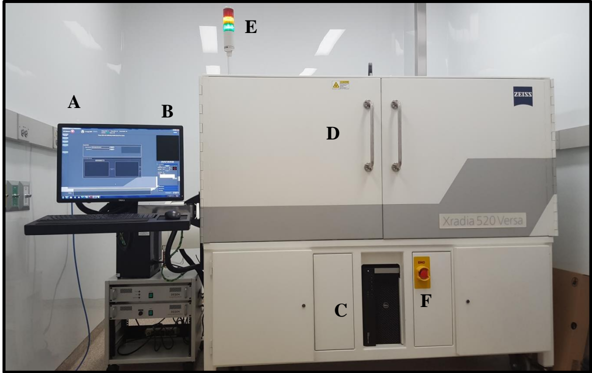
Figure 4. Setup of the Versa 520 scanner. Labels: A – Control computer display, B – Scanner interior video feed, C – Scanner control computer, D – Scanner cabinet, E – Status indicators, F – Emergency Reset.
